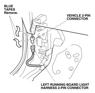
25. Plug the left running board light harness 2-pin connector into the vehicle 2-pin connector.
