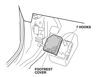
6. Remove the footrest (two flange nuts).
