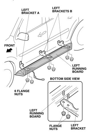
13. Align the front of the left running board with the left front door edge as shown.
