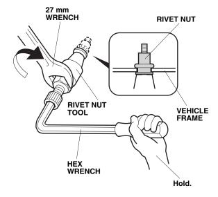
• Remove the rivet nut tool from the rivet nut by turning the hex wrench counterclockwise.
